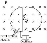
Suppose that a proton, injected by a source S at centre at time t = 0. Let us assume that at the instant the proton emerges into the centre gap from the first dee, the potential difference between des is reversed. Thus the proton again faces a negatively changed dee and is again accelerated. This process continues, the circulating proton always being in step with the oscillations of the dee potential, until the proton has spiraled out to the edge of the dee system.
